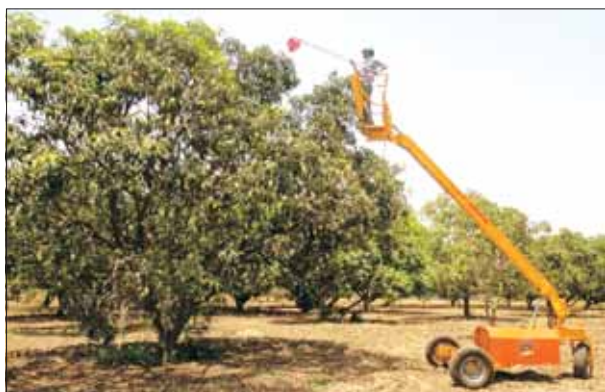
Self-propelled hydraulically hoisted platform for orchard management
