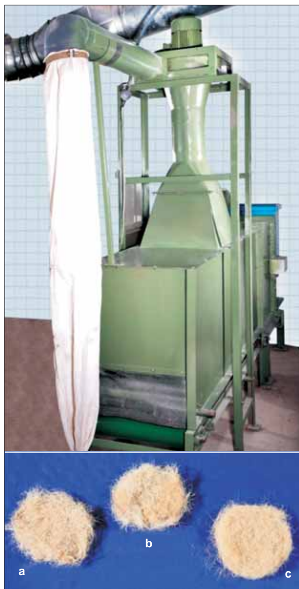
Coconut fibre segregator machine (top) and segregated coconut fibres – a, segregated coarse fibres; b, unsegregated (bulk) fibres; c, segregated fine fibres
