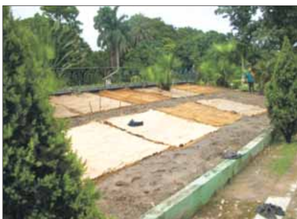
Jute-coconut fibre composite structured as backing material for making grass carpet
