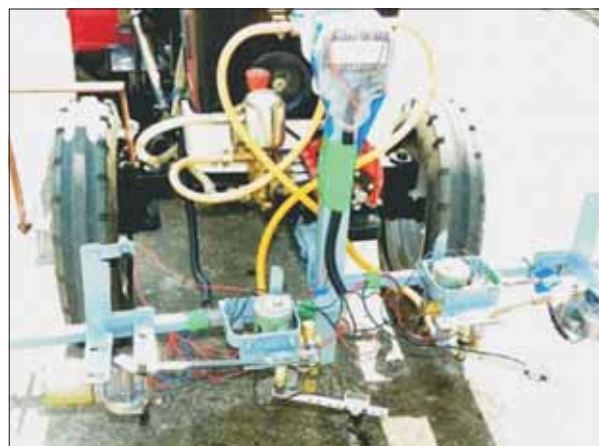
Colour sensor-based site-specific herbicide applicator
