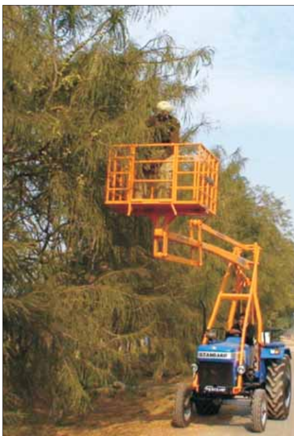
Tractor-mounted pick positioner for fruit harvesting and pruning
