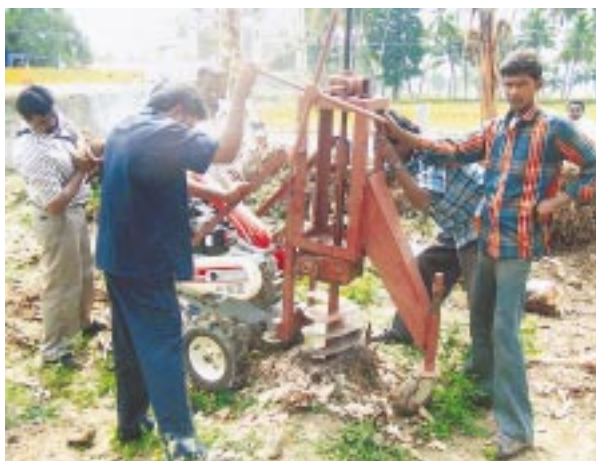
Desucking and clump removal equipment takes 5 min to remove big clump in dry condition and only 30 sec for small clump in wet condition
