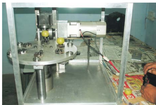
Continuous feed seed removal unit for use by the aonla processing industries
