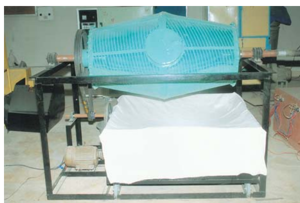
Thermal disinfestation set-up for pulses has a batch capacity of 100 kg
