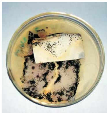
Antifungal property of control (left), 100% bulk nano (middle) and 100% nano-ZnO coated paper (right)
