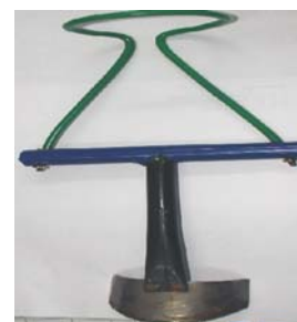
Banana-comb cutter facilitates cutting and separation of banana comb with minimum damage
