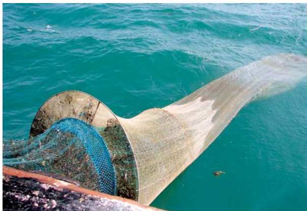
Operation of radial escapement device
