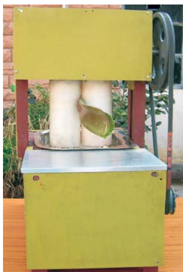
Crushing rollers are designed so that only gel is extracted
