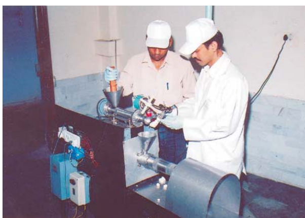
Continuous chhana ball making machine—it does not involve any contact of human hand during process
