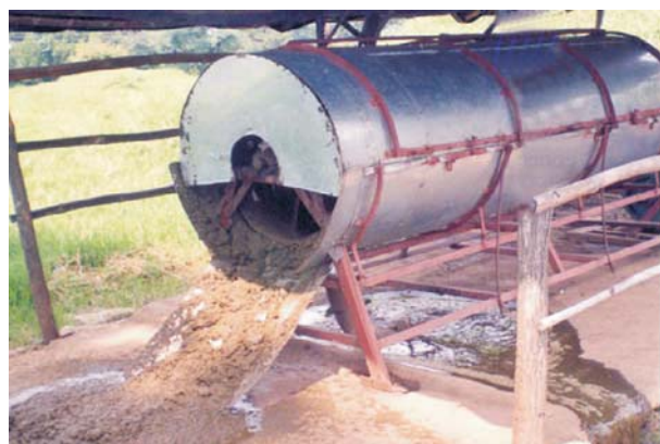
Biogas plant slurry dewatering machine
