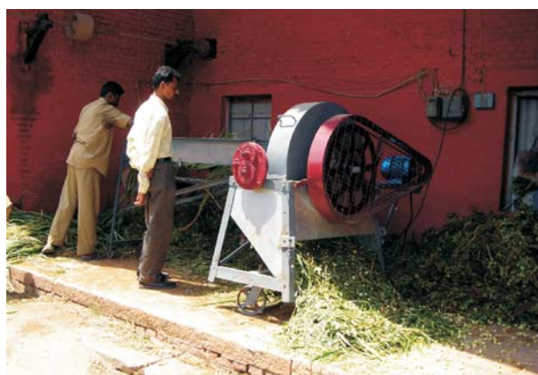
Safety gadgets ensure that operator's hands do not reach cutting machines
