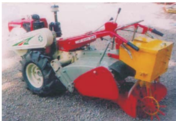
Power tiller-mounted earthing-cum-fertilizer applicator
