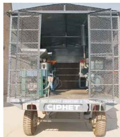
Mobile agro-processing unit, suitable for rural areas
