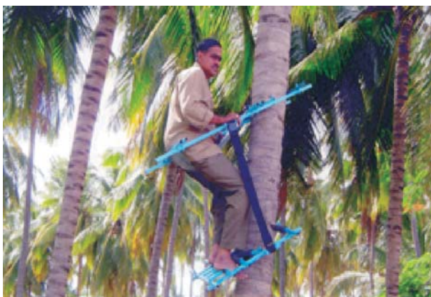
Tree climber helps operator to climb 10 m in 1.5 minutes
