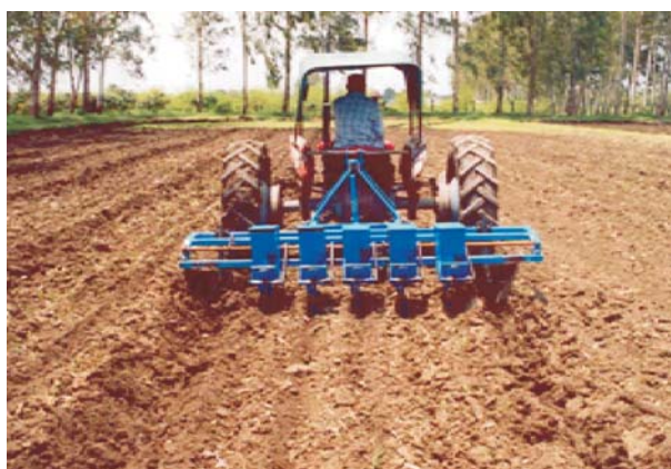
Tractor-mounted inclined-plate planter with raised-bed forming attachment for intercrop
