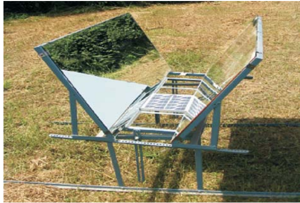
Concentrator for solar photovoltaic panel
