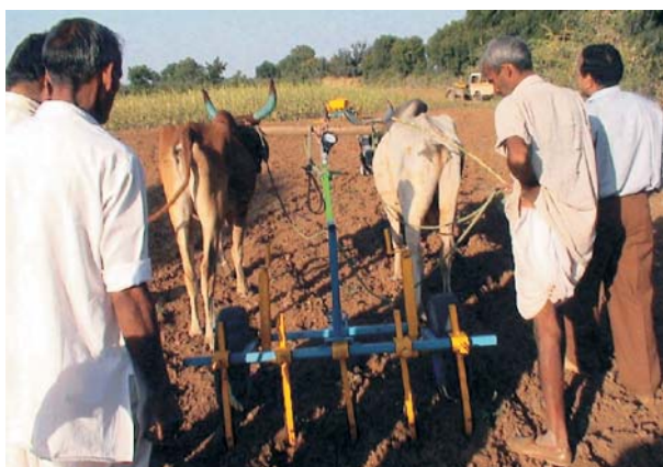
Animal-drawn tool carrier with attachment for tillage, seeding and weeding operations
