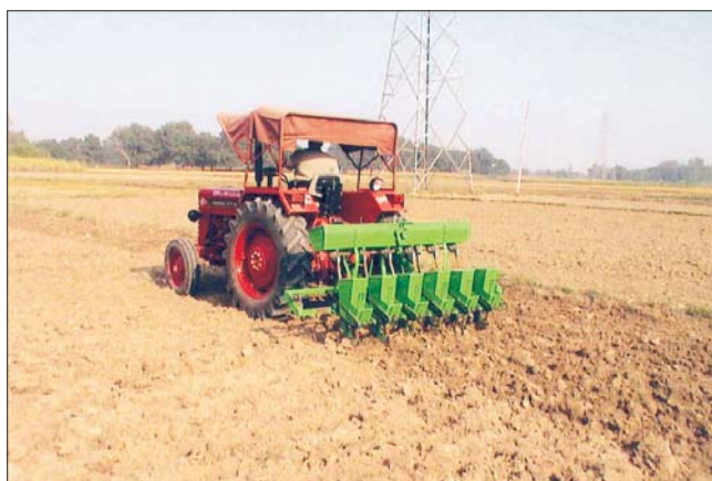
Inclined plate planter in operation
