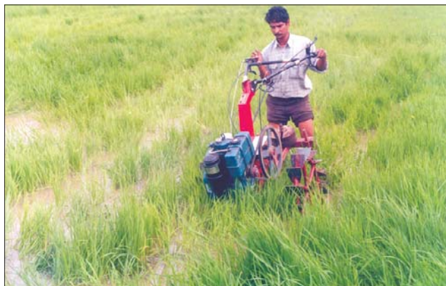
Field testing of self-propelled biasi cultivator
