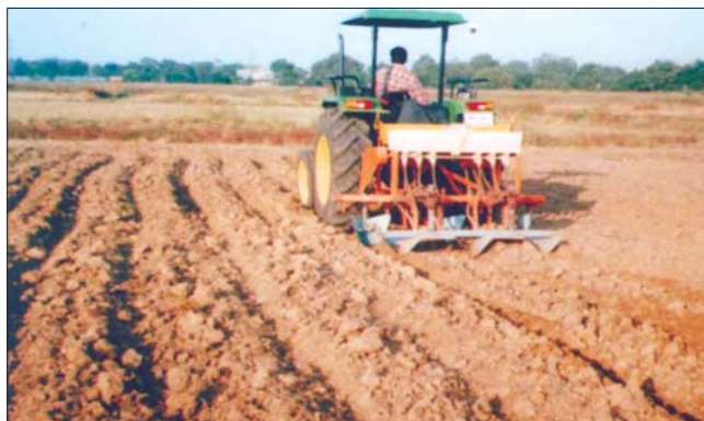
Tractor-drawn raised bed planter in working mode
