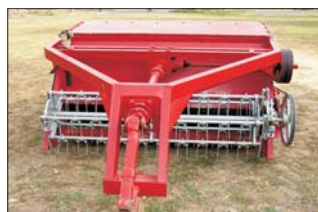
Modified cutter-bar type rice-straw chopper-cum-spreader
