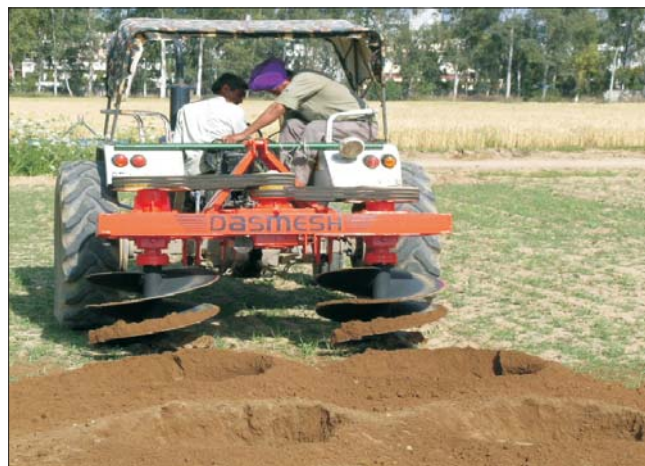
Twin-auger-digger sugarcane planter in operation
