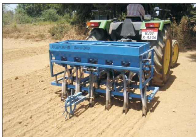
Tractor-mounted garlic planter. The observed seed rate during testing varied from 500 to 700 kg/ha depending on size of garlic cloves
