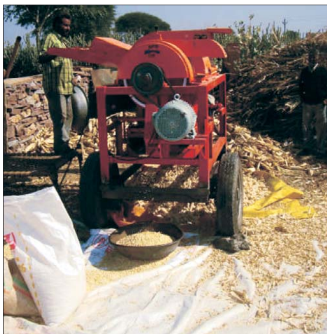
Whole crop maize thresher (5.5 kW capacity) in operation
