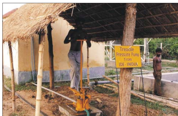
Treadle pressure pump operated with LEWA
