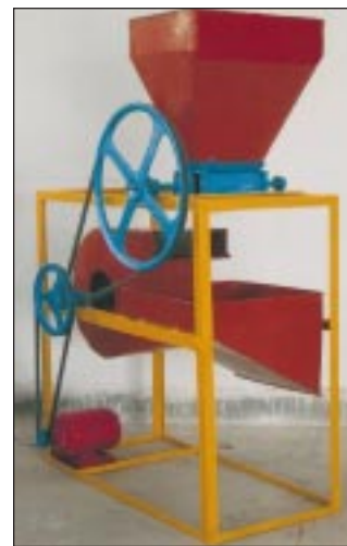
Hand-operated lac winnower for village level processing
