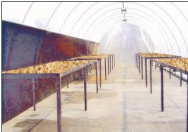
Walk-in type solar tunnel dryer installed in a farm for drying goose berry pulp
