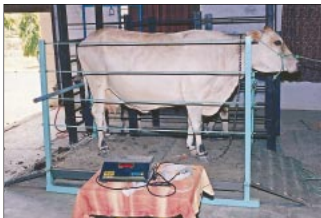
Portable electronic weighing machine for animals has the capacity of 1,500 kg (least count 1%)
