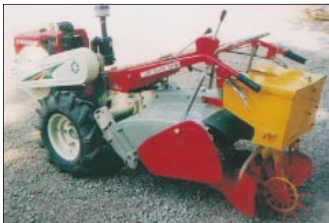
Power tiller mounted earthing-cum-fertilizer applicator for wide row sugarcane crop is developed by MPKV
