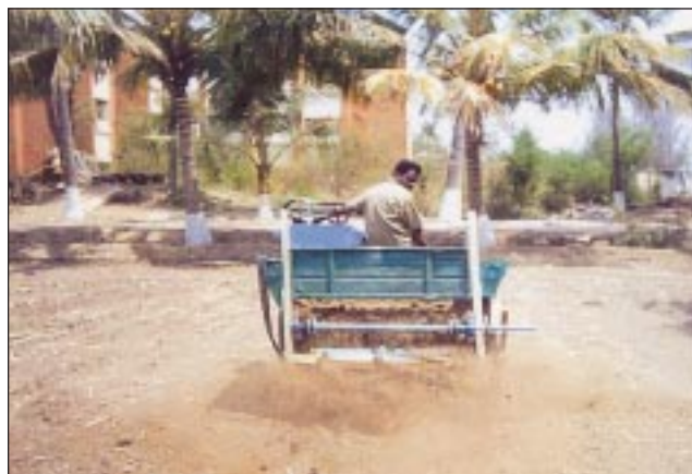
TNAU power tiller operated manure spreader. It has the field capacity of 0.62 ha/hr
