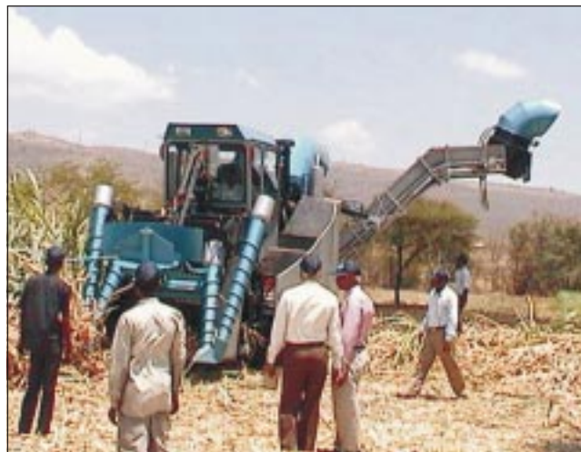
A prototype of indigenous chopper type sugarcane combine harvester developed to work even under adverse conditions
