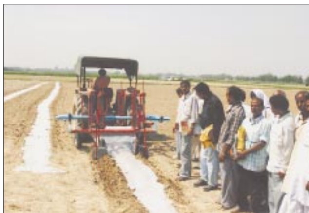
Plastic mulch laying machine. Plastic sheets from 5 to 30 micron thickness and up to 1,500 mm width can be used on the machine
