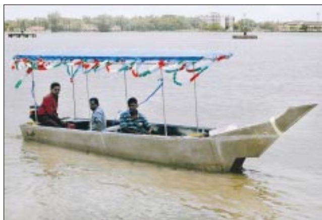
Prototype of the 5.20 m LoA aluminium alloy craft developed at the CIFT
