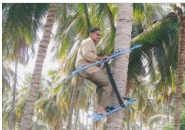
With tree climber the operator can safely climb a tree of 10 m height in 1.5 minutes
