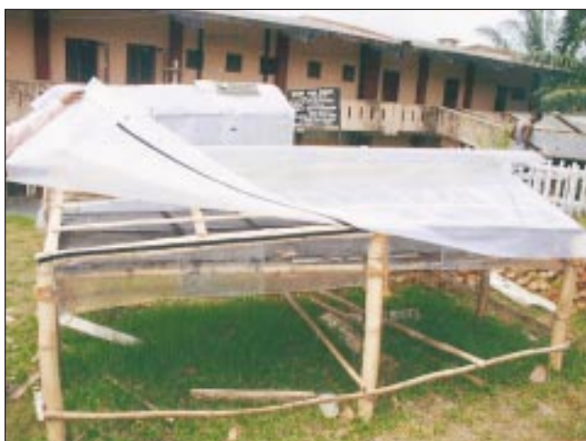
Low-cost solar dryer traps solar energy and improves copra quality
