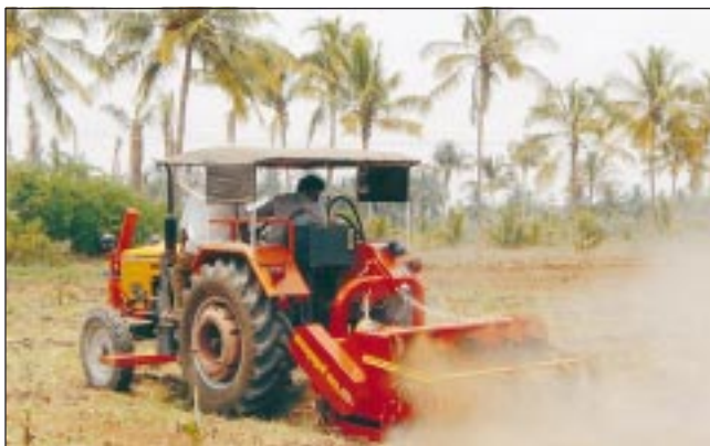
TNAU rotary field shredder for shredding sugarcane trash and crop residues
