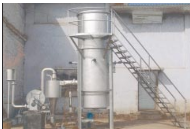
Open core biomass gasifier installed in an industry for chicory roasting
