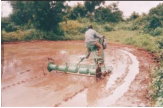
Riding-type rice-seeder. This seeder has been developed for sowing pre-germinated rice.
