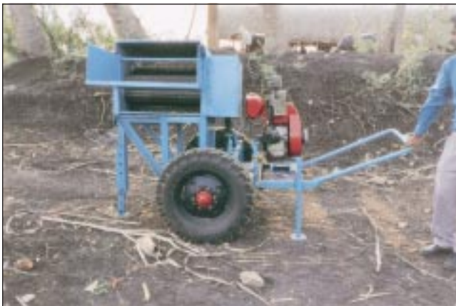
ANGRAU sugarcane leaf stripper. During trials at Hyderabad, its effective field capacity and fuel consumption were 1,300 kg/ha and 0.40-0.50 litre/hr.
