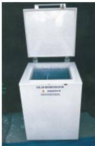
Solar refrigerator. This refrigerator has been used to store animal vaccines and other medicines in a village veterinary clinic.
