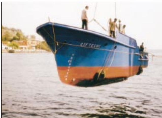
A fuel efficient deep sea multipurpose 15.5 m. OAL fishing vessel "CIFTECH -1" developed by CIFT, Kochi
