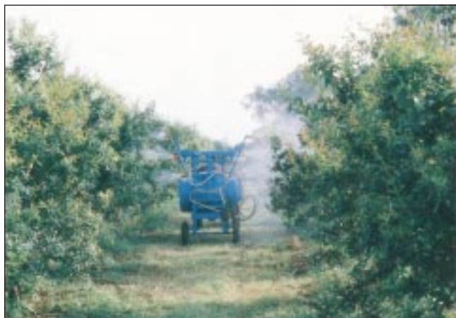
Orchard sprayer. Its field capacity is 0.80-0.90 ha/hr and gives droplets of 200-250 \mu m, and their density is 20-35 nos/sq cm.
