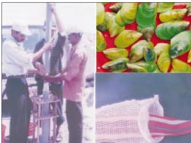
A semi-automated mussel seeding machine using flexible plastic strips and pre-stitched cotton tubing
