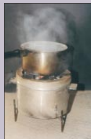
CIAE improved stove has been developed for biomass charred briquettes. About 0.5-kg briquettes can be fed at a time and that lasts around 1 hr.
