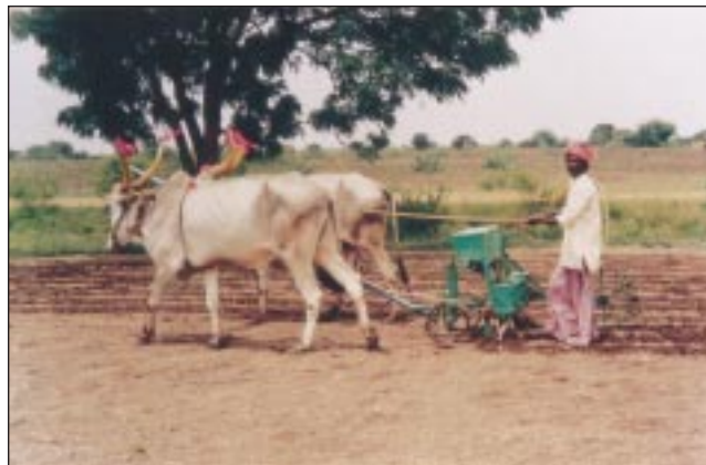
CIAE planter. Animal-drawn this machinery saves 64% on the operation cost compared to conventional method of sowing behind the country-plough with manual seed-dropping.
