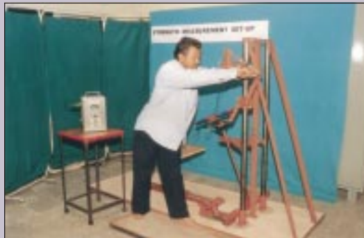
A strength measurement set-up for agricultural workers. Strength data of male as well as female agricultural workers have been collected to test working of the strength measuring set-up and to chalk-out protocol.
