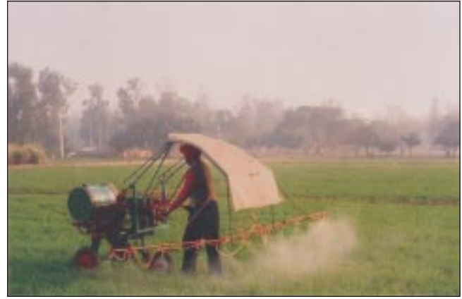
PAU walking-type sprayer. This could save 70-80% hr of labour and 45-50% in cost of operation compared to knapsack sprayer.
