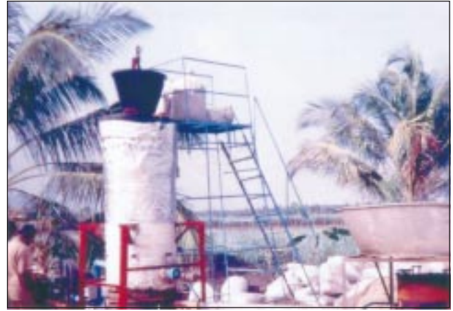
Bagasse-based gasifier. Developed an open-core gasifier of 700-mm internal diameter. This system has been installed at the site of the sugarcane-farmer for jaggery preparation. Its burner efficiency is 52% compared to 16% of the conventional system.
