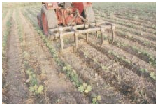
A tractor drawn 4-row weeder was developed. It can cover an area of 1.1 ha/hr.
