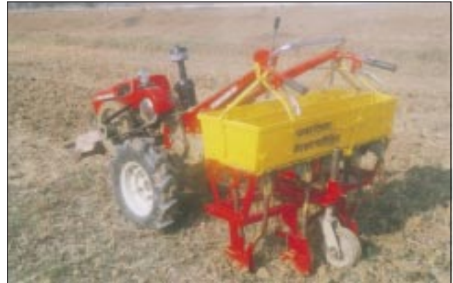
Power-tiller-operated zero-till drill. This NDUAT developed machine is suitable for 10-12-hp power-tiller. This saves 68% in time and 85% in cost of operation compared to conventional practice
