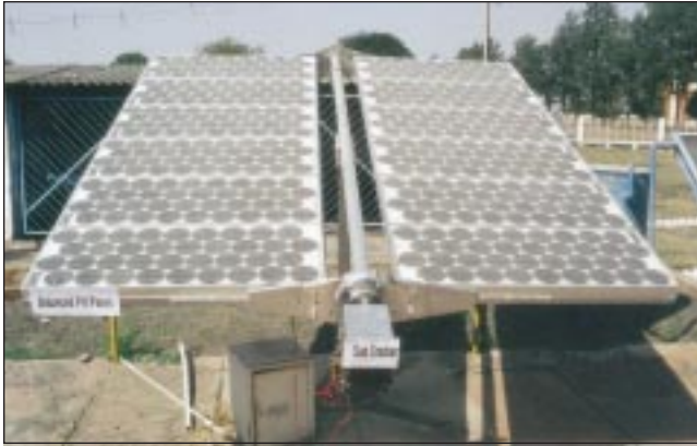
Modified solar tracking device. Sun tracker developed for 450 Wp SPV panel has been modified to adopt for 900 Wp SPV panel, to make it more reliable and user-friendly. The peak power output has been observed to be 660 W during noon time on a typical sunny day in summer.
