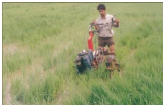
Two-row cultivator for biasi operation. This self-propelled cultivator has been developed for dry-seeded rice (broadcast/row seeded). Its field capacity is twice as much as that of animal-drawn, 2-bottom biasi plough and three times that of farmer's practice of single-bottom wedge plough.
