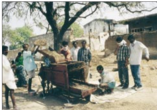
CRIDA castor sheller. Its performance was very satisfactory.
