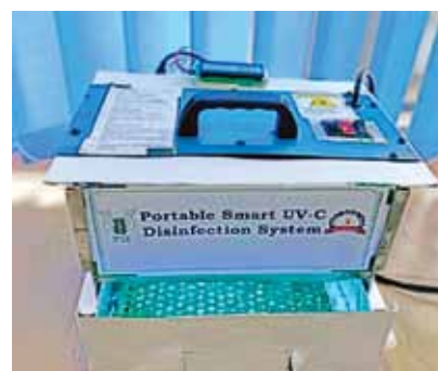
Portable smart ultraviolet-C disinfection system (UViC)
