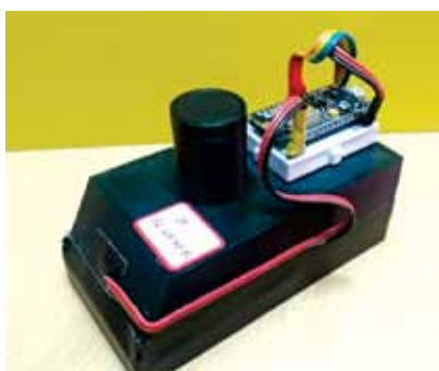
Automated amylose detection sensor system
