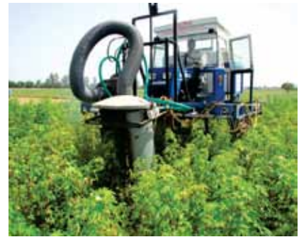
Sprayer equipped with electro-pneumatic system to control whitefly in cotton crop
