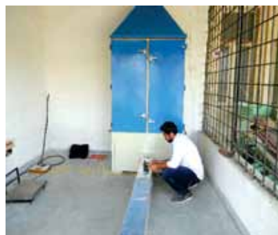
Solar assisted dryer for drying groundnut pods
