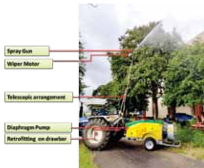
High pressure variable range sprayer
