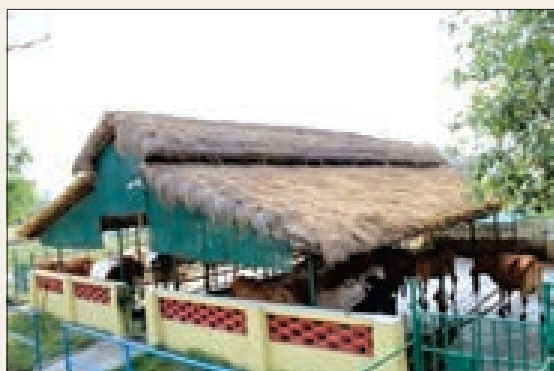
Thermo-comfortable thatched roof influences cow-shed's micro-environment
