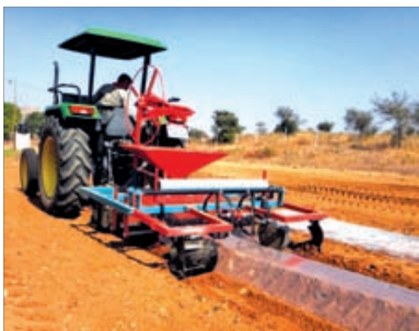
Tractor operated mulch cum drip laying and seedling planting machine
