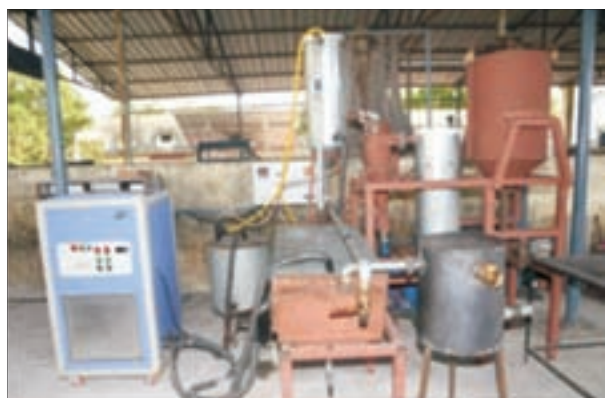
Fluidized bed reactor system for bio-oil production
