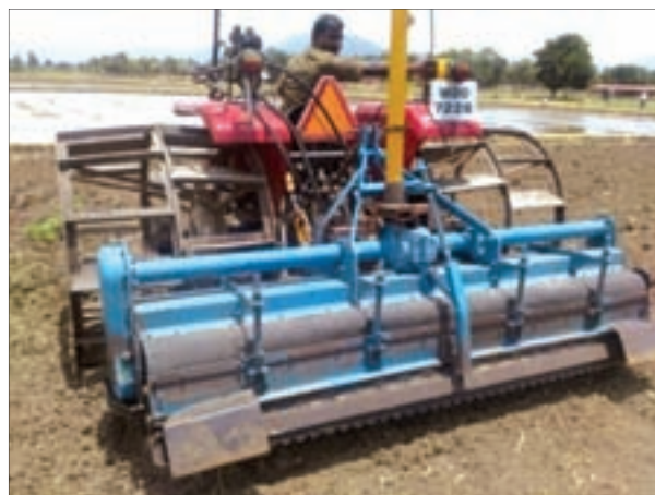
Tractor operated controlled level puddling system
