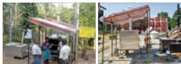
Indirect solar-biomass hybrid system for drying of spices
