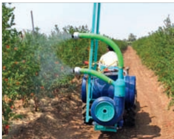
Variable rate vertical boom type air-assisted sprayer
