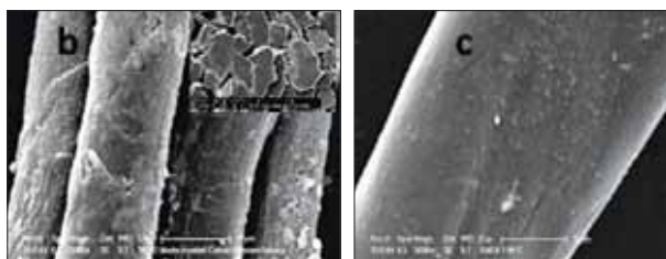
SEM images (a) control (b) nano-ZnO treated (c) nano-ZnO treated fabric sample after six cycles of washing. Inset (b) fibre cross section of treated fabric
