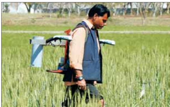
Variable rate urea application system, integrated with spectral reflectance based sensor
