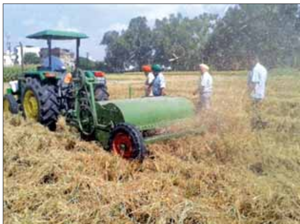
Loose straw chopper operating in the paddy field before wheat sowing
