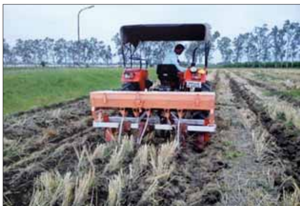
Seed-cum-fertilizer drill equipped with two stage fertilizer placement
